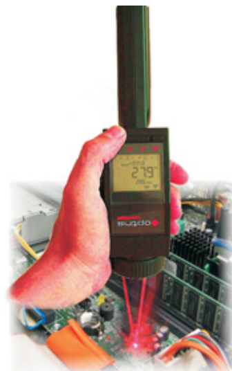
Highly accurate infrared temperature measurement with the optris LS of only mm small SMD components during a printed circuit board testing
